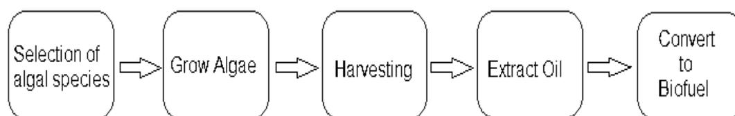
**Fig. 2** Steps of biodiesel production from algae.
