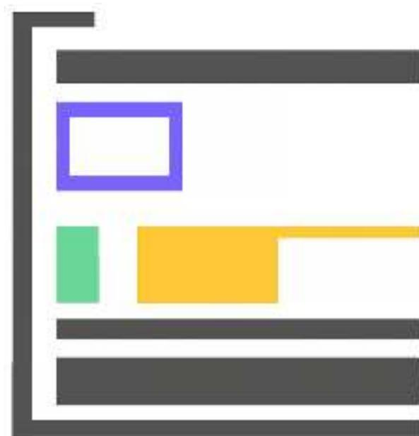
Fig. 13. Diagram of the layers of the housing package for Williams's *Portrait of John Samuel Holmes*. From top to bottom: glazing, spacers, spacers around the pastel, rigid backing boards, and barrier film that wraps around to the front of the glazing
