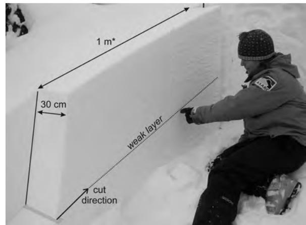
Figure 1. Example of a test column prepared for the PST. Weak layer is cut with a standard snow saw from the downslope end. ASARC photo.
