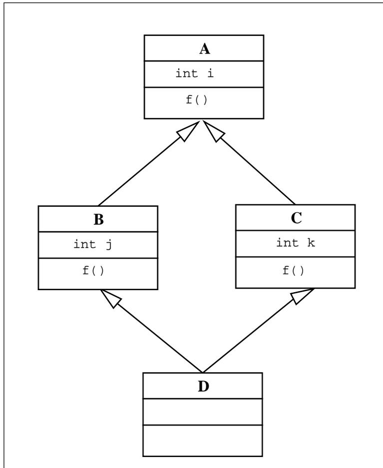
This UML 9.1 diagram shows four classes arranged in the diamond structure that creates the need for virtual inheritance. Both of the classes B and C inherit from class A. D multiply inherits
