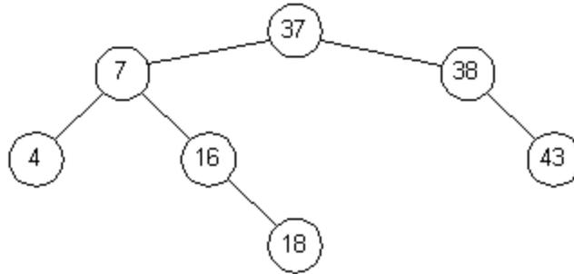
Figure 3-5: Binary Tree After Deleting Node 20
