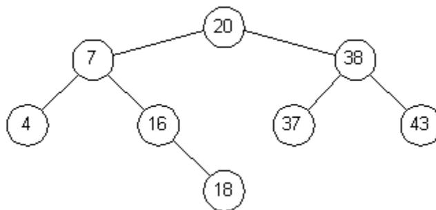
**Figure 3-4: Binary Tree After Adding Node 18**
