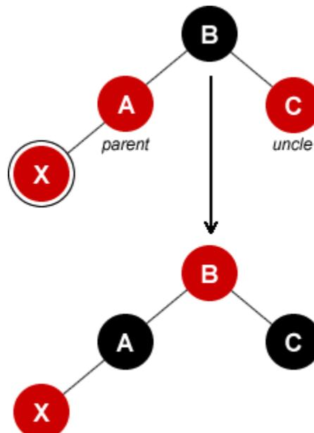
Figure 3-6: Insertion - Red Parent, Red Uncle
